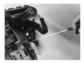
Press and hold the safety switch and then accelerator throttle to start the operation
