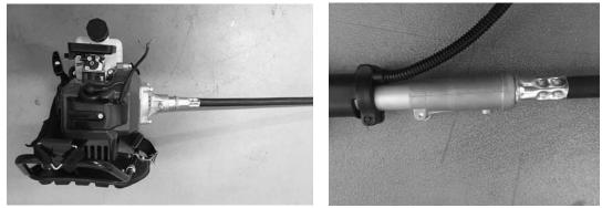
CAUTION: If the flexible tube is not inserted properly, the square end of the hose may not fit snugly in the drive shaft seal. Do not use force to avoid damage to the flexible shaft. Repeat the same procedure until the flexible shaft and hose are adjusted.
